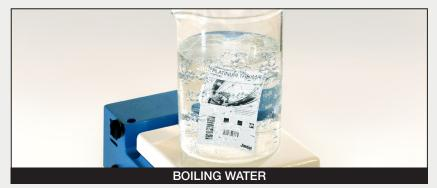
Boiling water exposure was tested by measuring white and black optical density after submersion in boiling tap water for 1 hour.
