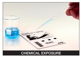
Two drops of a test solvent were applied to both the horizontal and vertical bar codes.
