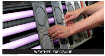
Platinum Thermal<sup>™</sup> Film was printed on a Zebra 140Xi4 thermal printer, then evaluated in a QUV Weatherometer according to ASTM, BS, and ISO standards. Test samples were exposed to varying conditions of ultraviolet radiation, moisture and heat.
