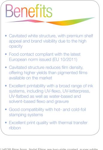
LH538 films from Jindal Films are two-side coated, super white opaque polypropylene label facestocks. They provide high whiteness and a high level of opacity due to Jindal Films' unique cavitation process.
