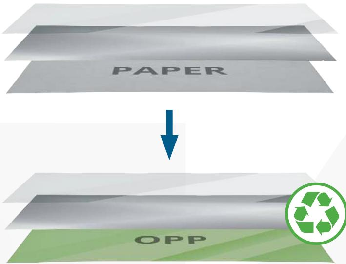
**Paper** can be substituted either with OPPalyte™ white films (MW647) or Bicor™ clear films with a matt-look (CSR). Using non heat sealable matt OPP will help for packaging efficiency while providing a paper finish aspect.
