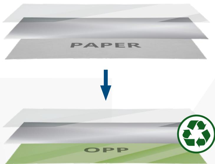
**Paper** can be substituted either with OPPalyte™ white films (SHH, ORH) or Bicor™ clear films with a matt-look (CSR). Using non heat sealable matt OPP will help for packaging efficiency while providing a paper finish aspect.
