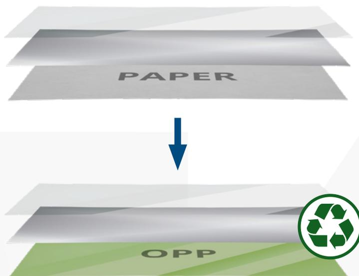
**Paper** can be substituted either with OPPalyte™ white films (SHH, ORH) or Bicolor™ clear films with a matt-look (CSR). Using non heat sealable matt OPP will help for packaging efficiency while providing a paper finish aspect.
