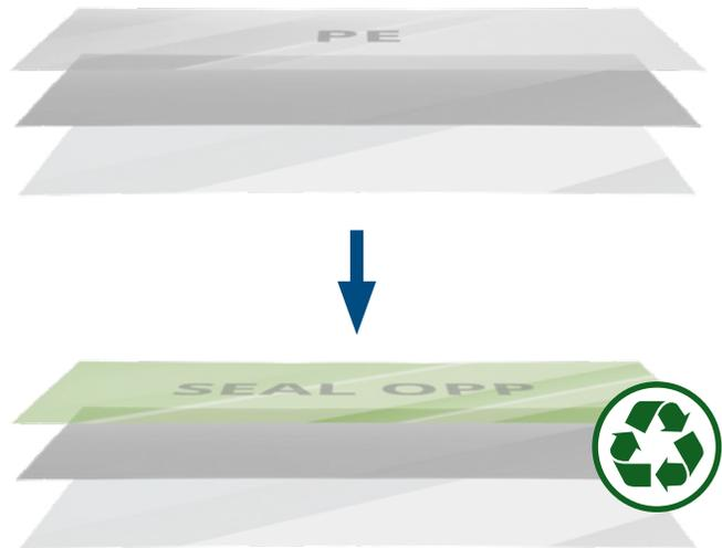
Jindal Films has developed specific Bicolor™ or Metallyte™ films with higher seal performance to partially close the gap with PE-based sealants. The latest generation of Bicolor Ultra Seal films (MB344US) delivers 6 times higher seal strength than most standard coex OPP films, with exceptional hot tack window and often with lower seal initiation temperatures (SIT) than most cast PP films.
